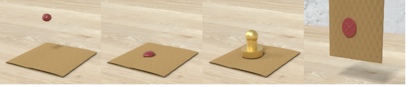
Fig. 2. Wax seal. Our distance-based model is robust under severe compression and large plastic deformations. Here, we press on top of a small dollop of wax to seal the letter. The wax remains adhesive after being squashed and is printed with an 'X' mark by the stamp. The wax is modeled with an energetically consistent von-Mises plasticity with StVK elasticity [7] within our optimization time integrator.
